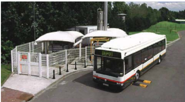
Bio-methane bus at refuelling site in Lille
